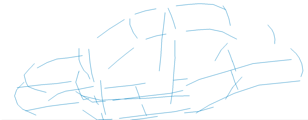
Fig3.: Equivalent beam modeling of the BIW
