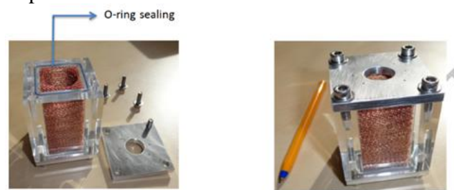
Figure 3: Schematic of a thermal management system based on a phase change material with a copper mesh [80]
