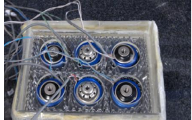
Figure 6: Battery pack with ethylene glycol and aluminum mesh in the research of Azizi and Sadramli [79].
