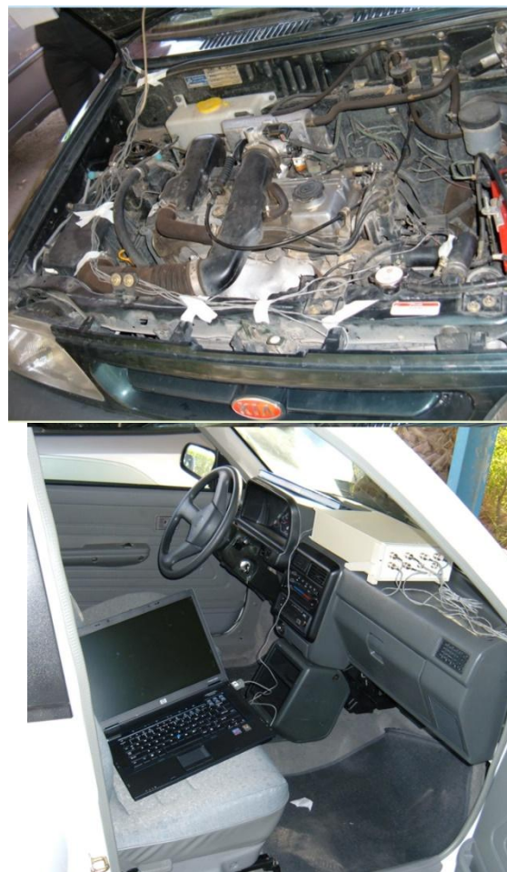
Figure 7: The data acquisition system and temperature sensors
