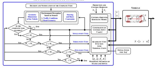
Figure 3: Overall structure of the proposed integrated planning and control system.
