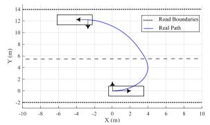
Figure 6: The real path in single-point turn task.
