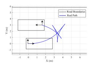
**Figure 10:** The real path in Five-point turn task.
