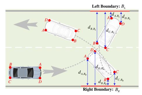
Figure 4: Schematic of the collision avoidance constraints.
