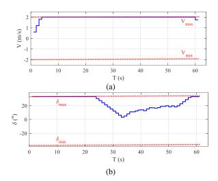
Figure 7: The control inputs in single-point turn task. (a) Velocity, (b) Front steering angle.
