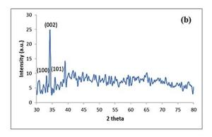
**Figure 3:** The XRD patterns of the (a) ZnO seed layer (b) well-aligned ZnO NRs arrays.
