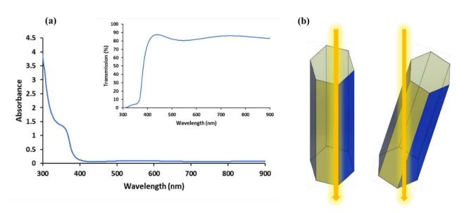
**Figure 4:** (a) Absorption spectra of the ZnO NRs. The inset shows the transmission spectra of the ZnO NRs. (b) the optical path traversing through nanorods
