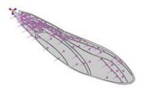
**Figure 8:** Uniform pressure loading and boundary condition
