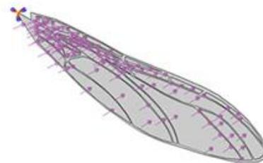
**Figure 8:** Uniform pressure loading and boundary condition
