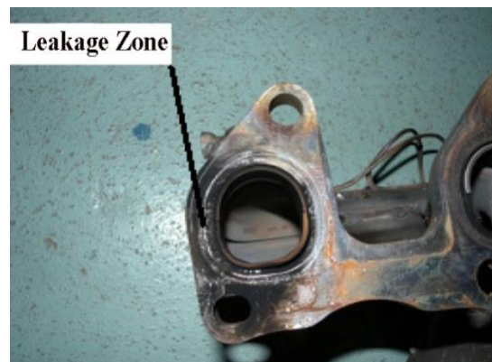
Figure 14: Evidence of gas leakage on the manifold exhaust
