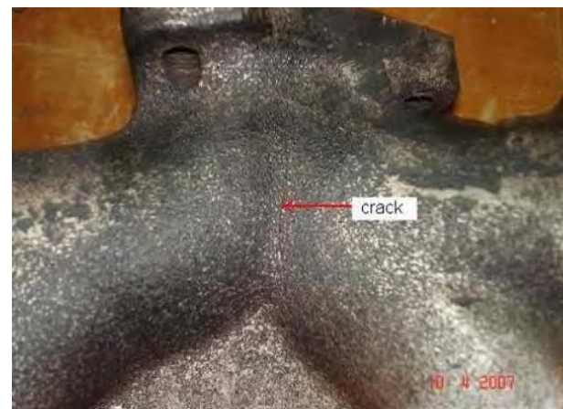
Figure 18: The cracked exhaust manifold [38]
