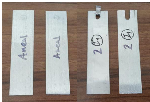
Figure 4: Failure modes. Left: IF failure mode - Right: PF failure mode
