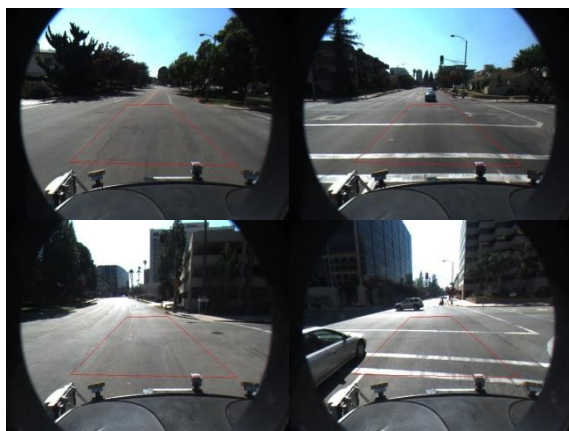
Figure 12: Lane detection when no lane presents in the image of Cordova 1 (top row) and Cordova 2 (bottom row)
