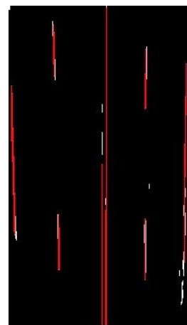
Figure 7: Red lines are fitted on the points in a thresholded image using Probabilistic Hough Transform.
