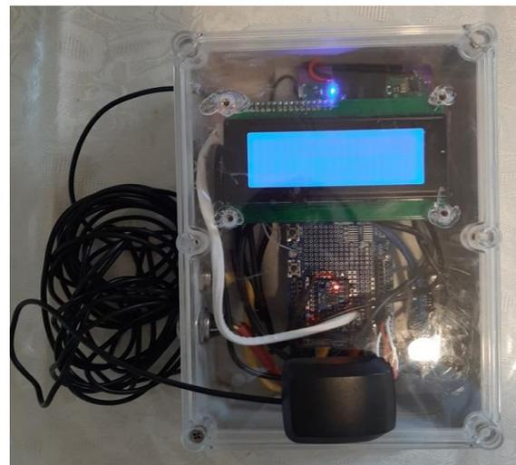
**Figure 3:** Data acquisition system
