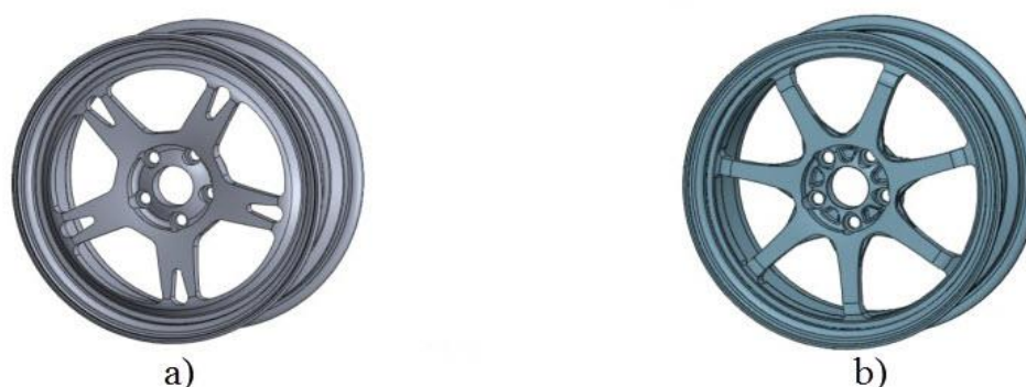
Figure 28: a) Optimized Wheel, b) Wheel in the market
