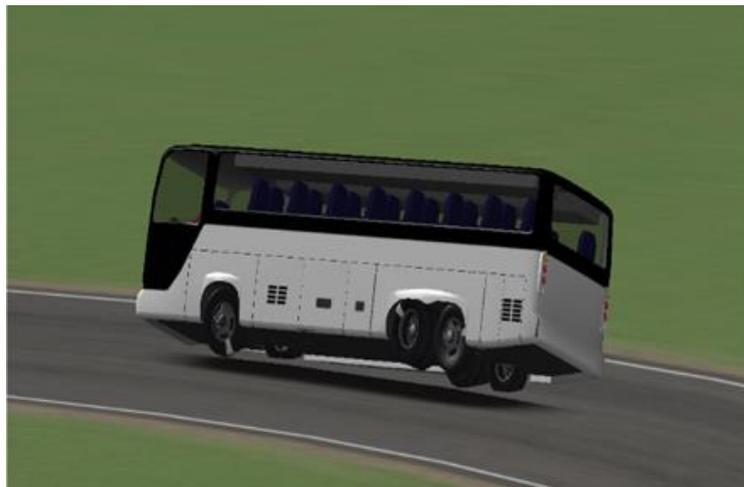
Figure 6: Triaxial bus while cornering and rollover in TruckSim software
