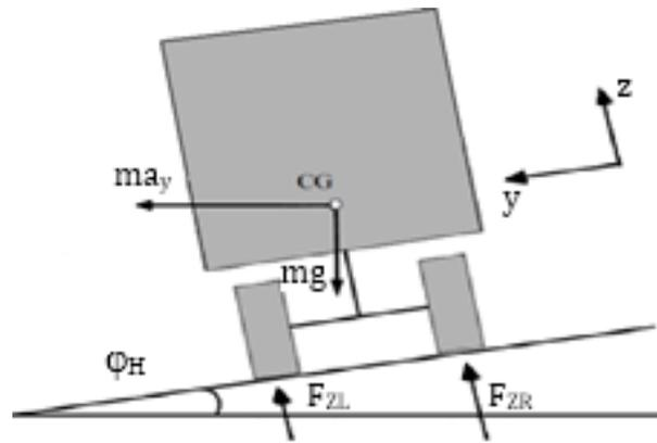
Figure 2: Vertical forces acting on the car
