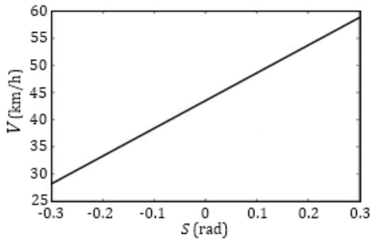
Figure 16: Vehicle speed diagram versus road bank
