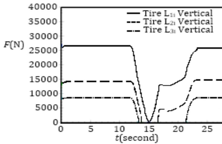
Figure 7: In turn tires vertical forces while rollover
