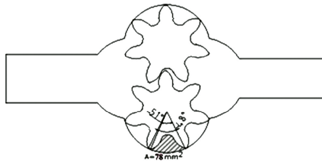
Fig8. Geometry of the old gear oil pump (7 teeth)
