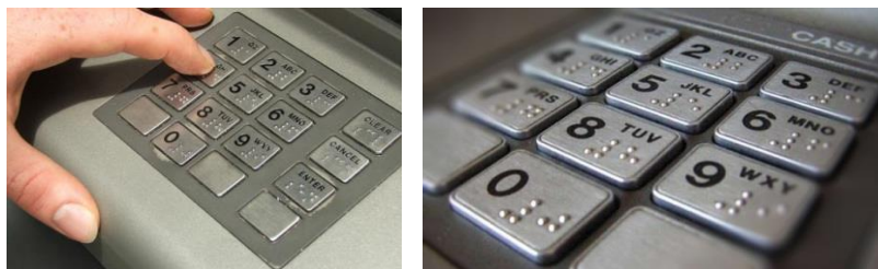
Fig1. Texture applied to ATM for blind person [source: www.zidbits.com ]
