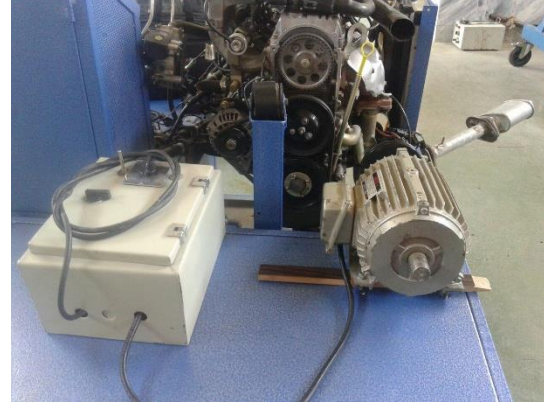
Figure 1: Motor setup, electric motor and inverter
